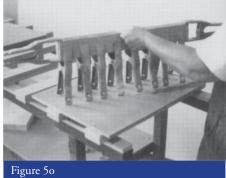
clamped up in eight to ten minutes or before adhesive begins to cure! Spring clamps should be set 3" on center. Failure to use enough clamps may result in inferior edge joints.
