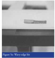
Using the wavy-edge system by Porter Cable or Pinske<sup>®</sup> Edge or Bosch® A-Line, provides excellent vertical alignment of seam and a stronger seam due to the increased surface area for bonding. This method eliminates the need for "biscuits" and has proven to be just as strong.
